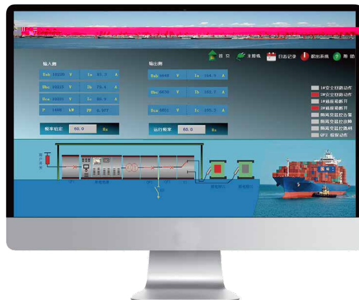
Shore Power Monitoring System
